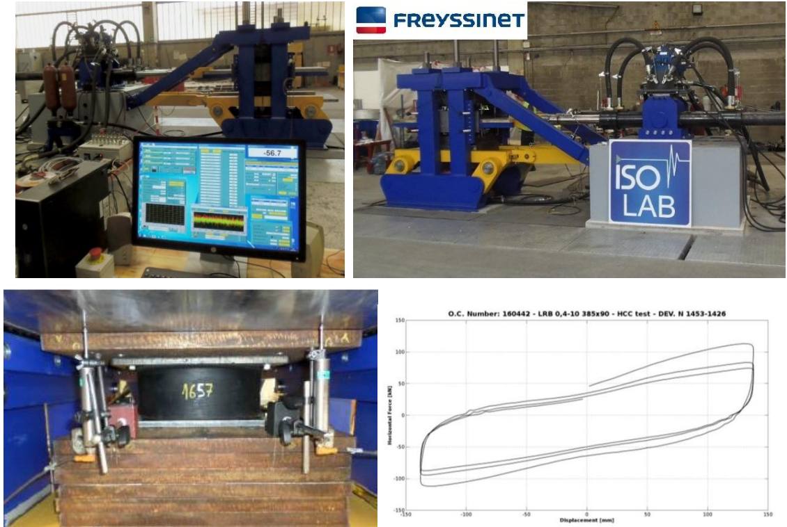
Figure 10: Isolab testing equipment for LRT Jakarta LRB and test performed
